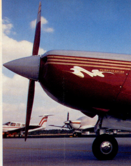
On Mod Works' Pursuit 221 ES, a modified 231 cowl housing a tuned-induction Continental IO-360 engine.
